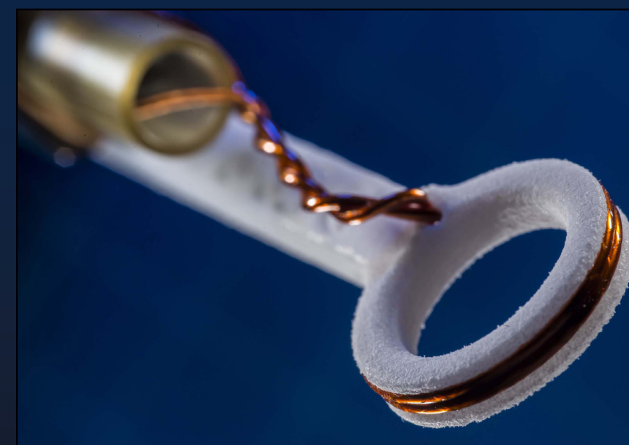
Magnetic coil wound around a 3-D-printed frame
