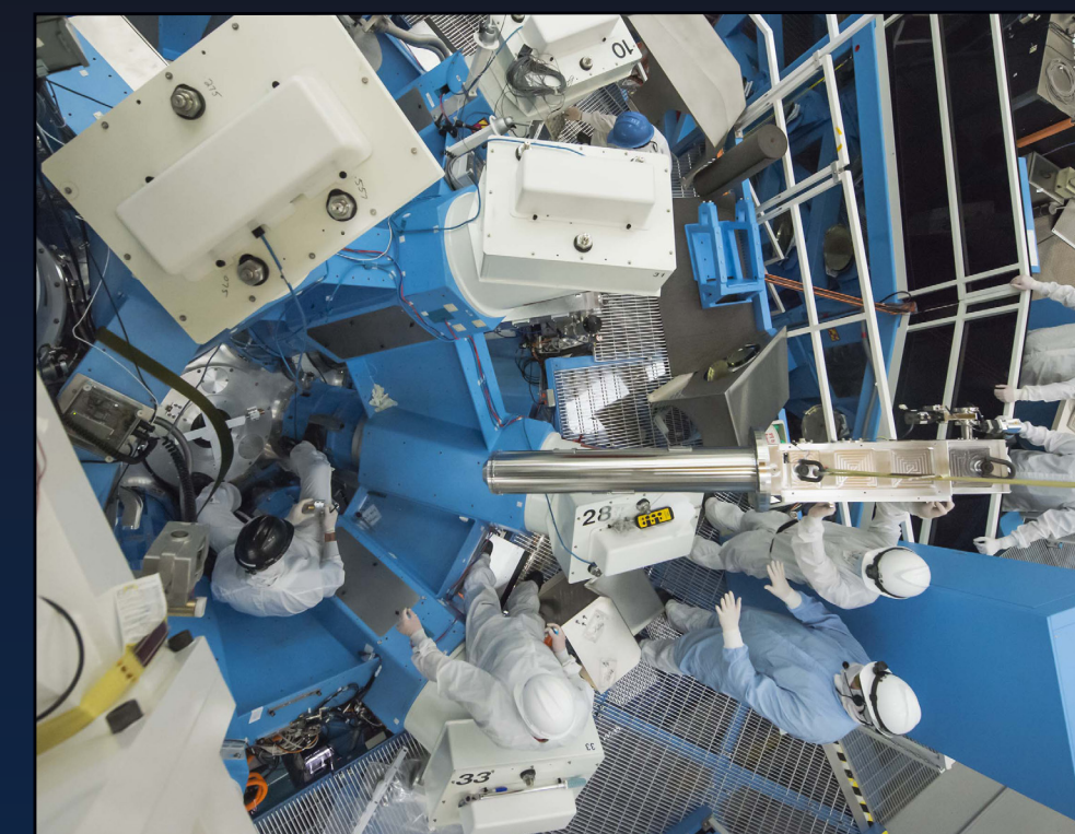
NTD assembly being lowered into the target chamber during installation in June 2013
